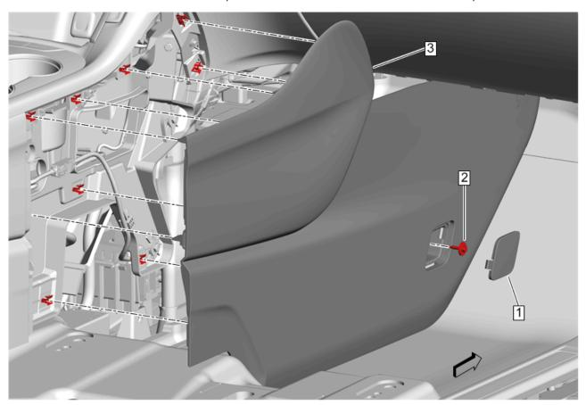
2. Remove the right side front floor console extension panels. Refer to Front Floor Console Extension Panel Replacement - Right Side in SI.
