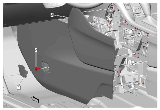
1. Remove the left side front floor console extension panels. Refer to Front Floor Console Extension Panel Replacement - Left Side in SI.
