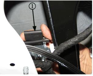
4. Locate the front and rear window regulator clamp rubber inserts and remove them from the regulator.
