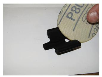
5. Using 80 grit sandpaper, lightly sand the inside surfaces of each rubber insert.
