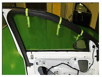
3. After detaching the window from the regulator, manually move the window to its full up position, and securely tape to the window frame.
