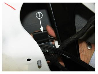
Important: When installing the inserts, ensure they are positioned with the wing to the inboard side, at each location.
