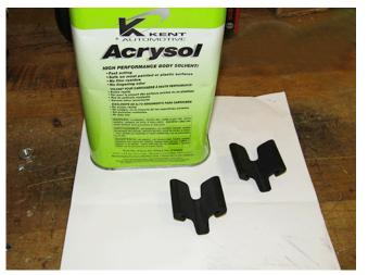
**6.** Using Kent Automotive Acrysol,®\* or equivalent cleaner, wipe the sanded surfaces of each insert.
