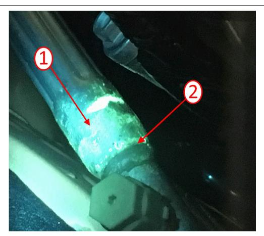
This condition may be caused by a refrigerant leak (1) at the weld (2) on the A/C heat exchanger line or compressor hose.
