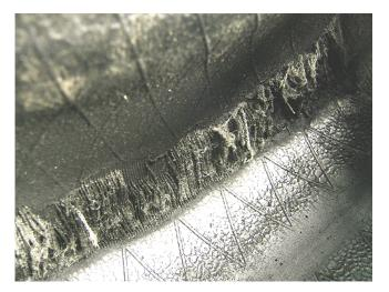
• This tire was damaged by extended driving with little or no air, same as the tire previously shown. This photo shows the inside view. Shredding of the inside may not always be accompanied by obvious exterior damage.
