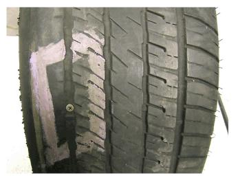
• This tire has two non-warrantable conditions. The tire is badly worn on the inside shoulder (over extended mileage) and has suffered air leakage from a screw still in the tread.
