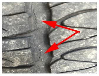
Some tire weathering and superficial cracking is normal. Tires should not be replaced under the New Vehicle Warranty for this condition.
