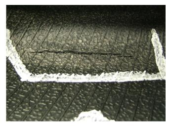
• This example of common road damage is called a *rim-pinch*. The damage to the tire is caused by the tire folding and contacting the rim and the pavement. Frequently this type of damage will cause a sidewall bulge/bubble when the tire is re-inflated, due to the air attempting to leak from the interna sidewall breakage. It is common for the rim-pinch damage to be visible only from the inside of the tire. A typical tear to the sidewall from this type of damage is shown.
