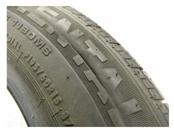
• This tire shows sidewall damage extending completely around the tire. This damage is the result of extended driving on a tire that is completely flat. The
