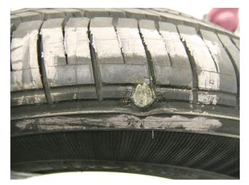
• This tire was returned for air leakage. The source of the air leakage is a tire repair plug installed in a non-approved portion of the tire. This tire has road hazard damage.
