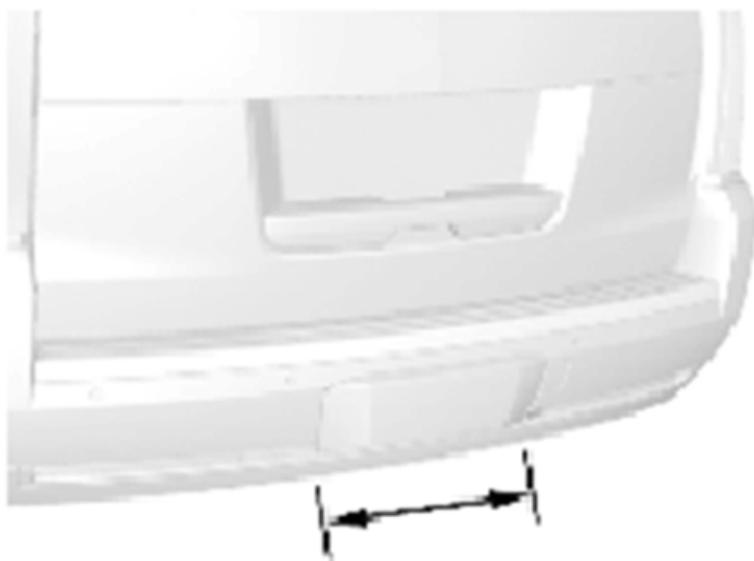
3. To operate, kick your foot straight up in one swift motion under the center of the rear bumper, then pull it back. There are two antenna's located in the rear bumper fascia which both must be triggered for the system to detect a kick. During the kick, your foot and shin must come within 6.5 inches (16.5 cm) of the rear fascia for both antenna's to be triggered and detect the kick, as shown below (1).
