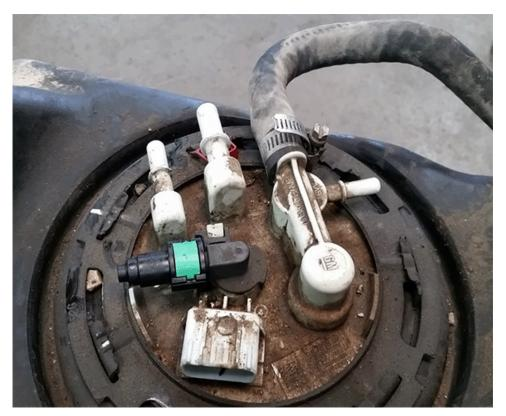
3. Measure the Fuel Tank Fill Vent hose 5 ½" from the end at the fuel pump module and cut with hose cutters as seen below (2).
