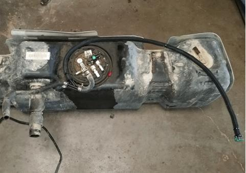
7. Remove the original fuel balance pump line from the pump tube (7) Refer to Plastic Collar Quick Connect Fitting Service. Doc Id# 2147646 and cross member (8) as seen below.
