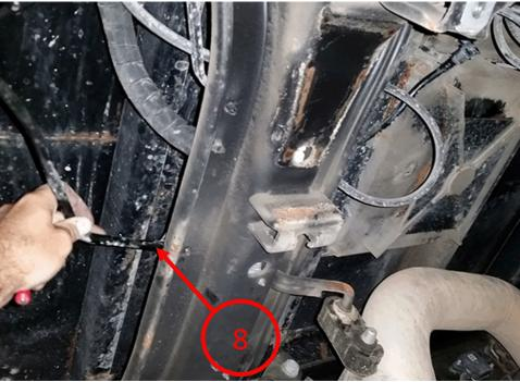
8. Remove plastic clip (9) seen below from fuel balance pump line and place clip back into hole in cross member.
