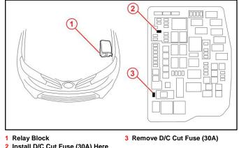
Install D/C Cut Fuse (30A) Here (Original Location)
