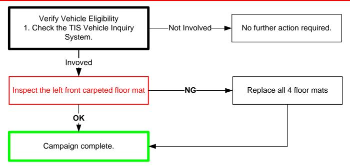
NOTE: All-weather floor mats are *not* involved in this LSC. If all-weather floor mats are installed in the vehicle and the carpeted floor mat is NG place the new mats in the trunk. DO NOT install the carpeted mats on top of or under the all-weather mats.
