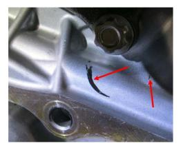
• Take note of how the sealant on the removed cover forms an additional "seal" when it becomes displaced into the chamfer around the inside edge of the case's machined surface at assembly.
