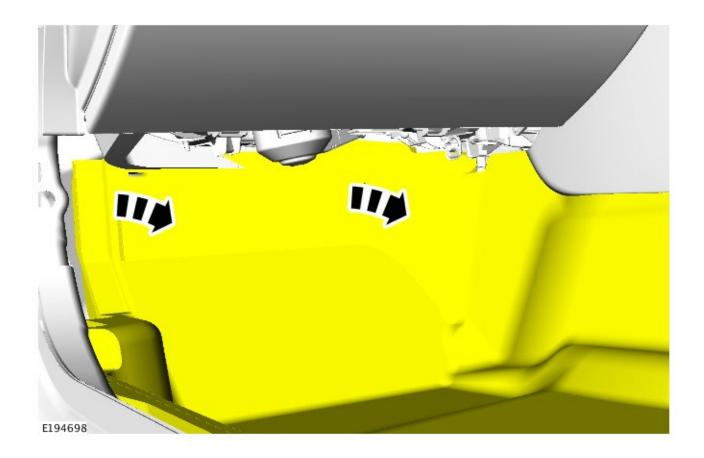
**9.** Using a syringe or similar tool, remove any standing water located in the lower 'A' pillar using the access hole shown.
