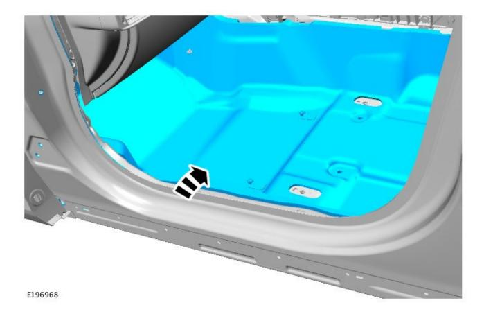
**11.** Install the fasteners to the front left carpet.
