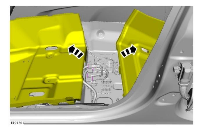
$\ensuremath{\textbf{15.}}$  Position the heater vent to one side to access the floor pan/ground terminals.
