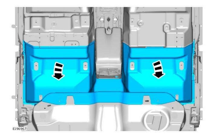
7. Install the rear carpets fasteners.
