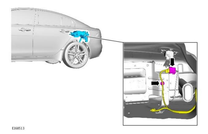
$\ensuremath{\textbf{4.}}$  Remove the evaporative emission canister assembly.
