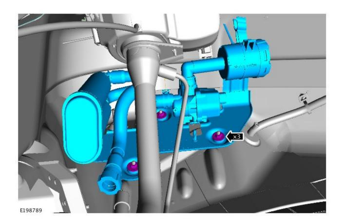
6. NOTE: The evaporative emission canister hose fasteners must be reused to install the new evaporative emission canister hose.
