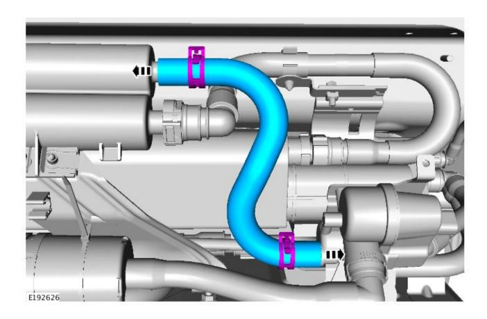
$\textbf{6.} \ \ \text{Install the evaporative emission can ister hose fasteners into their final position.}$
