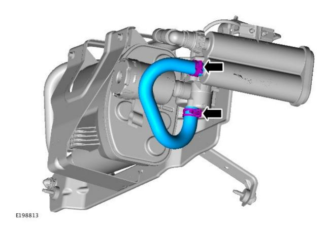
$\boldsymbol{8.}$  Install the evaporative emission canister assembly.
