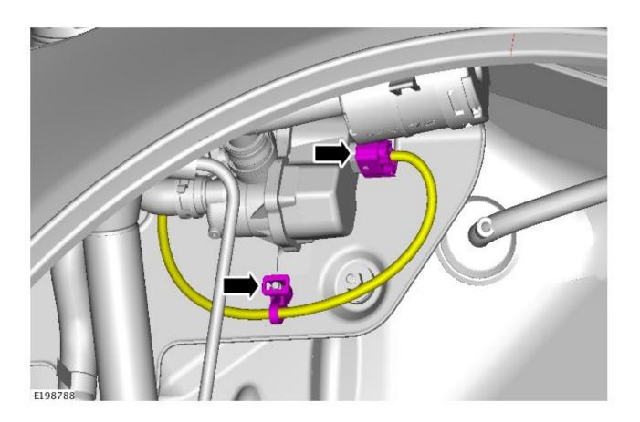
$\textbf{5.} \ \ \text{Remove the evaporative emission can ister assembly}.$
