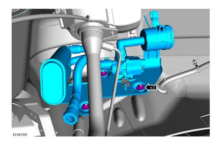
10. Install the connector and fastener.
