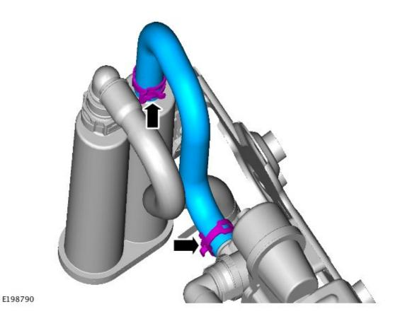
$\textbf{9.} \ \ \textbf{Install the evaporative emission can ister assembly.}$
