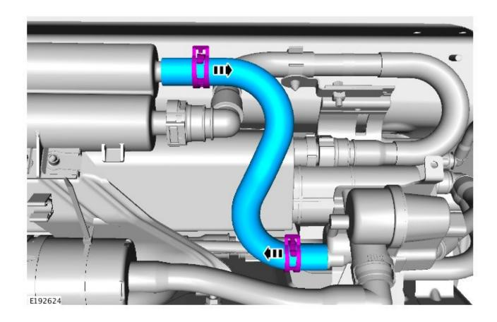
3. NOTE: The evaporative emission canister hose fasteners must be reused to install the new evaporative emission canister hose.
