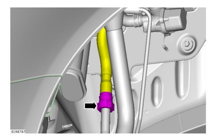
**4.** Remove the connector and fastener.
