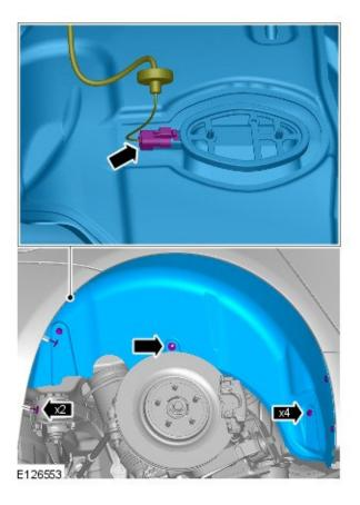
3. NOTE: The evaporative emission canister hose fasteners must be reused to install the new evaporative emission canister hose.
