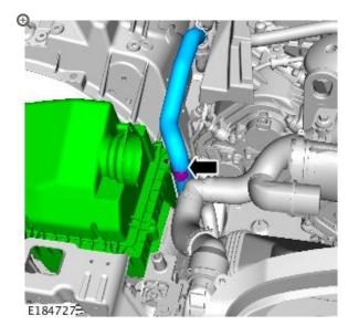
Check that the fir tree clip for the coolant hose is installed and located and secure on the right-hand air cleaner.
