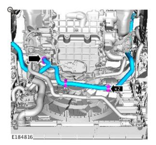
Release the coolant hose retaining clips.
