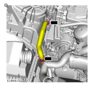
Release the coolant hose retaining clips and position to one side.
