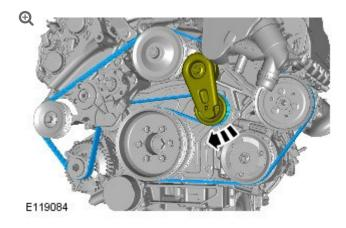
Remove the accessory drive belt from the idler pulley.
