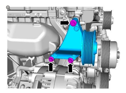
Install the new accessory drive idler pulley and bracket assembly.
