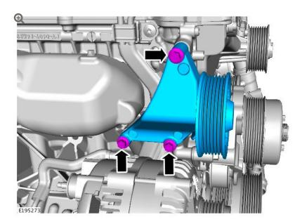
Remove the accessory drive idler pulley and bracket assembly.
