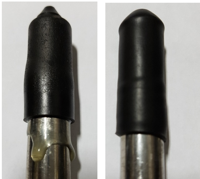
Figure 7 Incorrectly installed vent caps. Left image shows too much heat applied. Right image shows insufficient heat applied.
