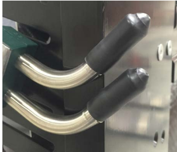
Figure 2 New heat shrink PRD vent caps in place. Production caps will be red, for higher visibility.
