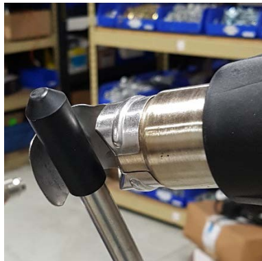
Figure 5 Using a hook accessory is another acceptable installation tool.
