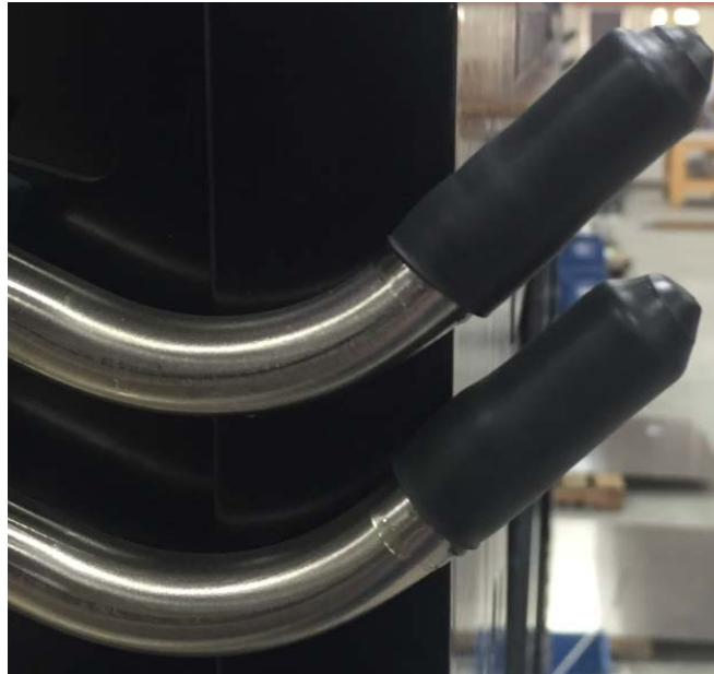
Figure 6 Correctly installed vent caps.
