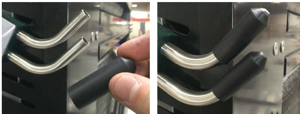
Figure 3 Vent cap installed prior to heating.
