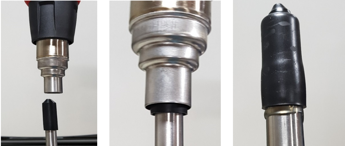
Figure 4 Installation using reducer nozzle.
