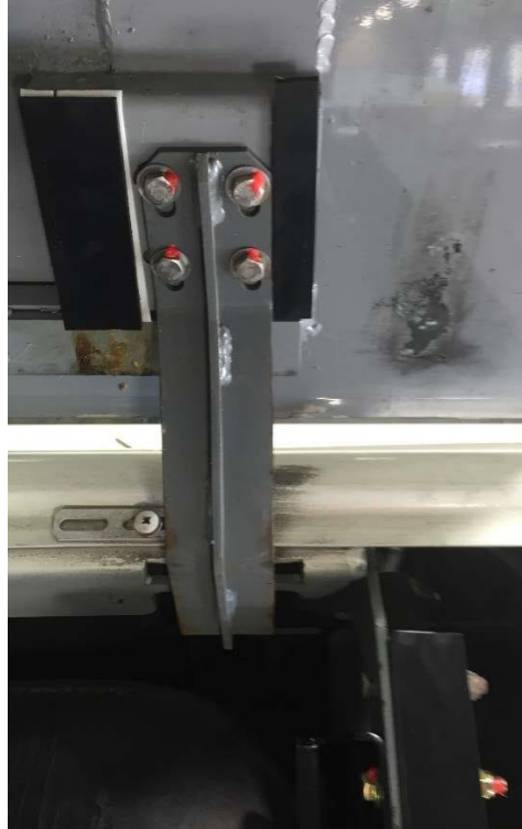
Figure 4 Location of rubber strips on doors. There should be two strips on either side of the hinge for a total of 8 pieces for each pair of doors.
