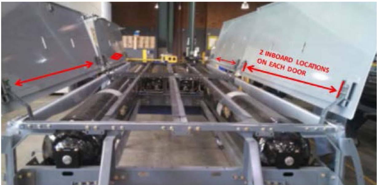
Figure 3 Small rubber strips at the door hinges may also be affected by adhesive failure.
