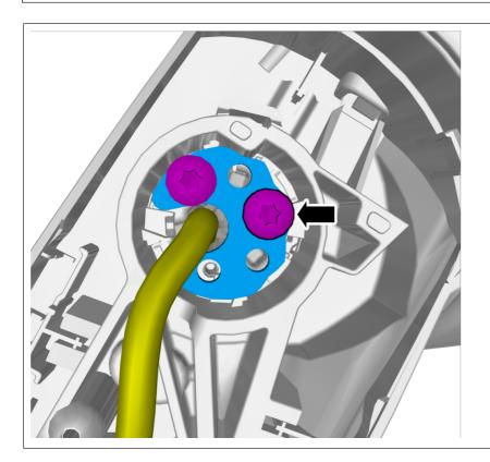
Add washer if screw reaches bottom of the hole when tightening.
