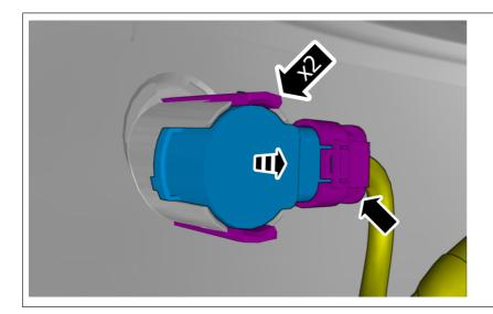
Disconnect the connector. Release the catches. Remove the marked part.
