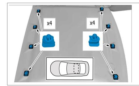
Note! Make sure that the mating faces are at a minimum temperature of 20°C.
