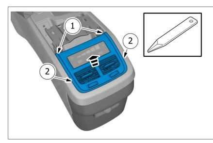
**Use:** Interior trim remover Remove the part carefully Remove the marked part.
