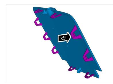
Note! The graphic shows the back of the component before removal.
