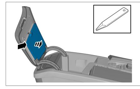
**Use:** Interior trim remover Remove the part carefully Remove the marked part. TJ 31491 Page 5 ( 7 )
