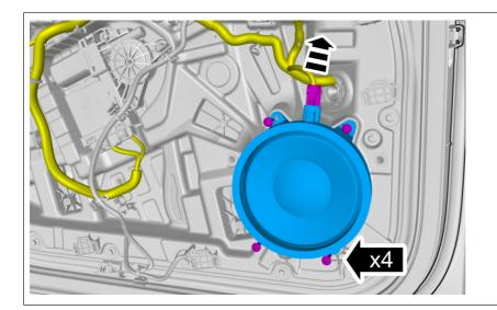
Disconnect the connector. Remove the screws.
