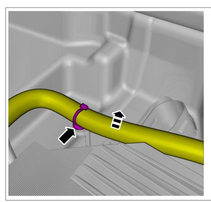
Remove the cable harness clips.
