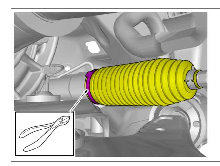
Remove the marked part. On both sides.
