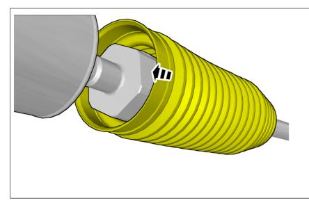
Install the marked component. On both sides.
