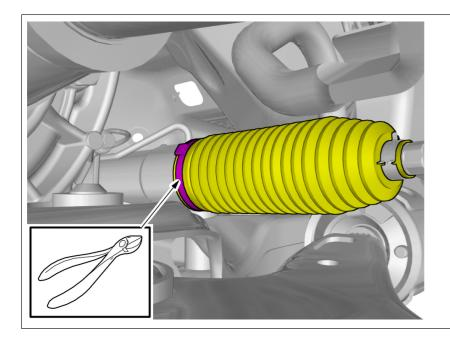
Install the marked component. On both sides.
