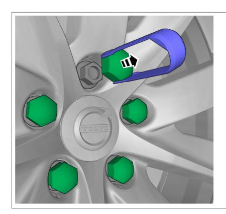
Remove the marked part. On both sides.
