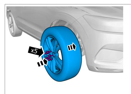
Install the marked component. Install the screws.
