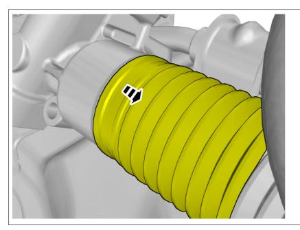
Fold marked part to one side. On both sides.
