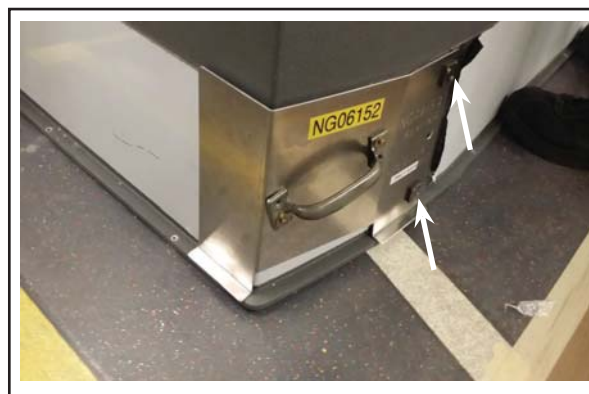
Figure 2 - Drilling Two Holes with NG06152 Drilling Jig in Curb Side Wheelhouse Kick-Plate
