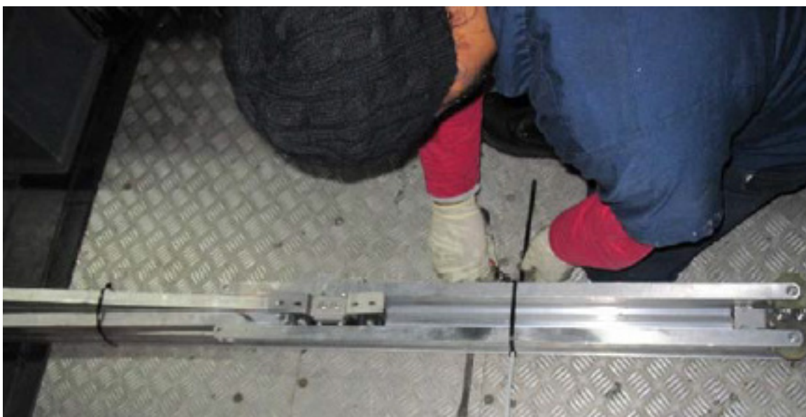
Figure 13 - Secure the Stabilizer Arms
