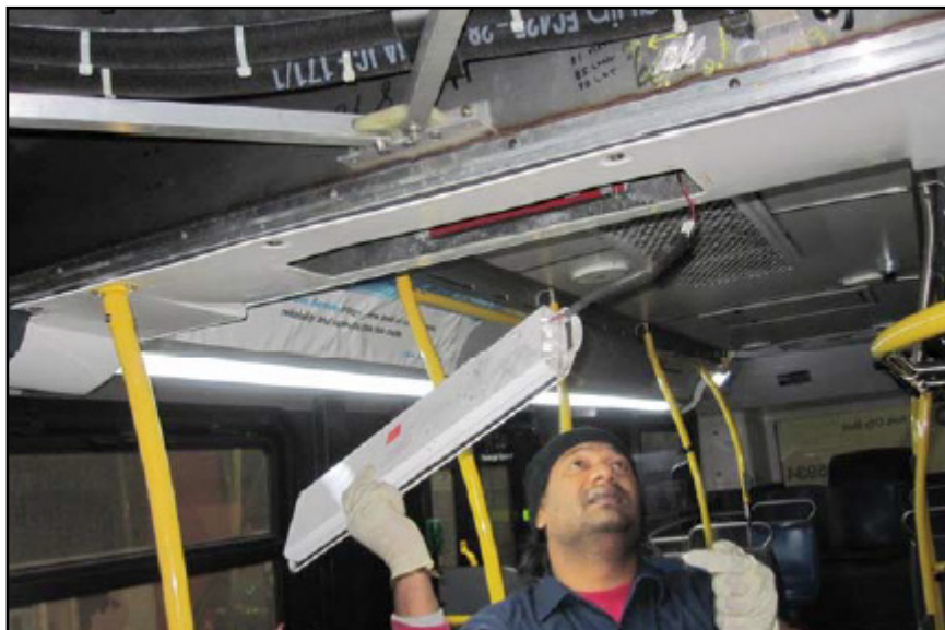
Figure 2 - Remove the Bulkhead Light
