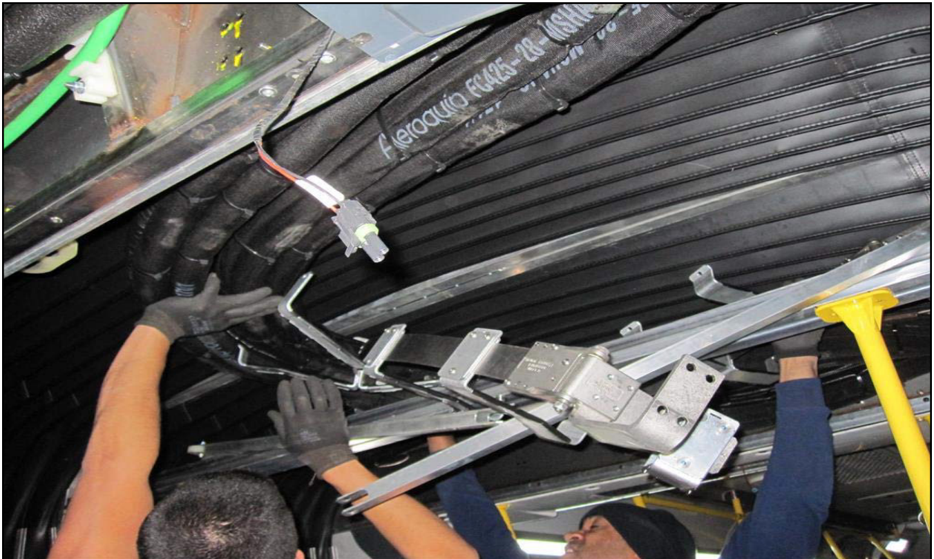
Figure 5 - Remove the EGS While Lifting the Cables and Hoses (New EGS Shown)
