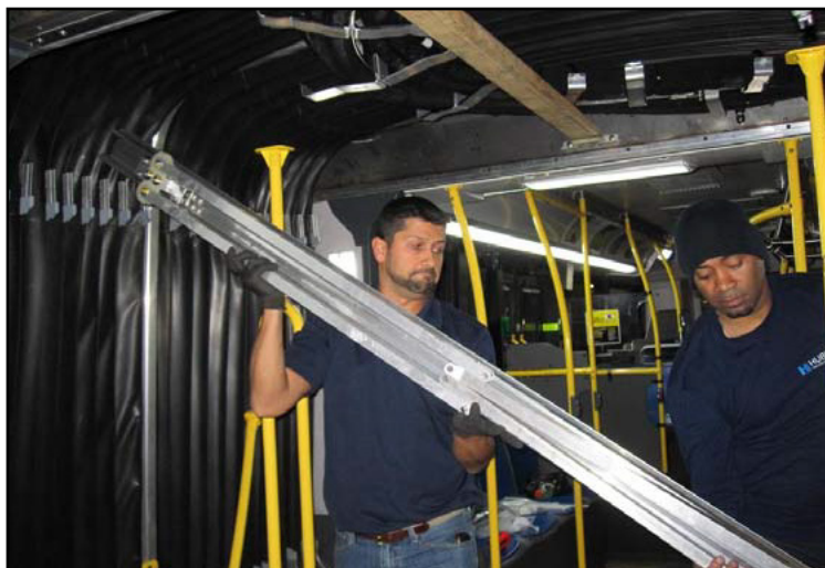
Figure 11 - Remove the Stabilizer Arms and Guiding Profile Assembly
