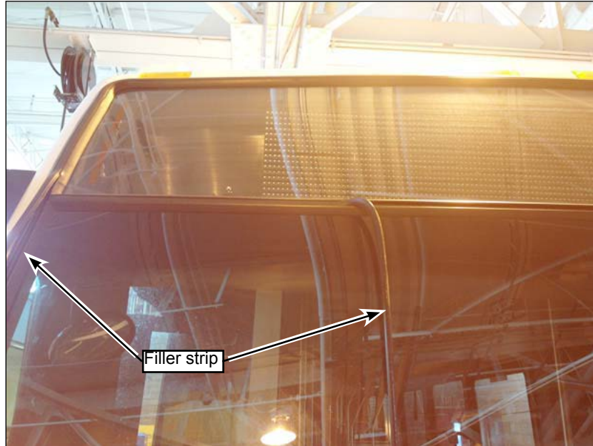
Figure 11 - Remove Inner Strip of Windshield Gasket and Windshield
