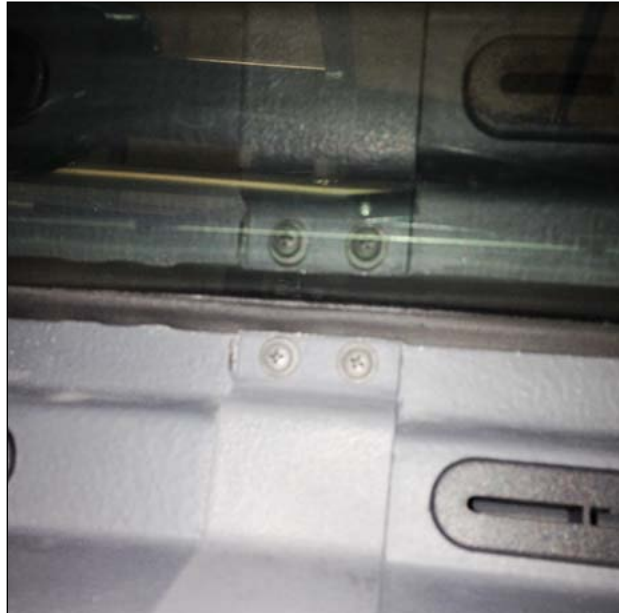
Figure 17 - Remove Dash Screws
