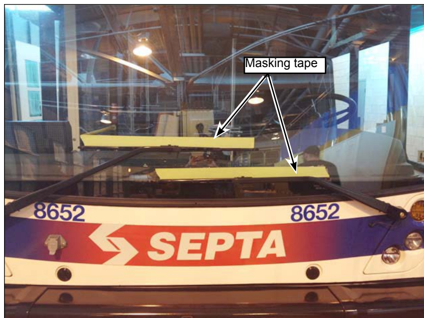
Figure 36 - Install Wiper Arms
