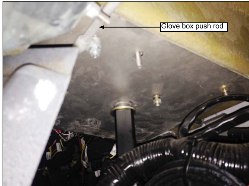
Figure 25 - Install Nuts and Glove Box Push Rod
