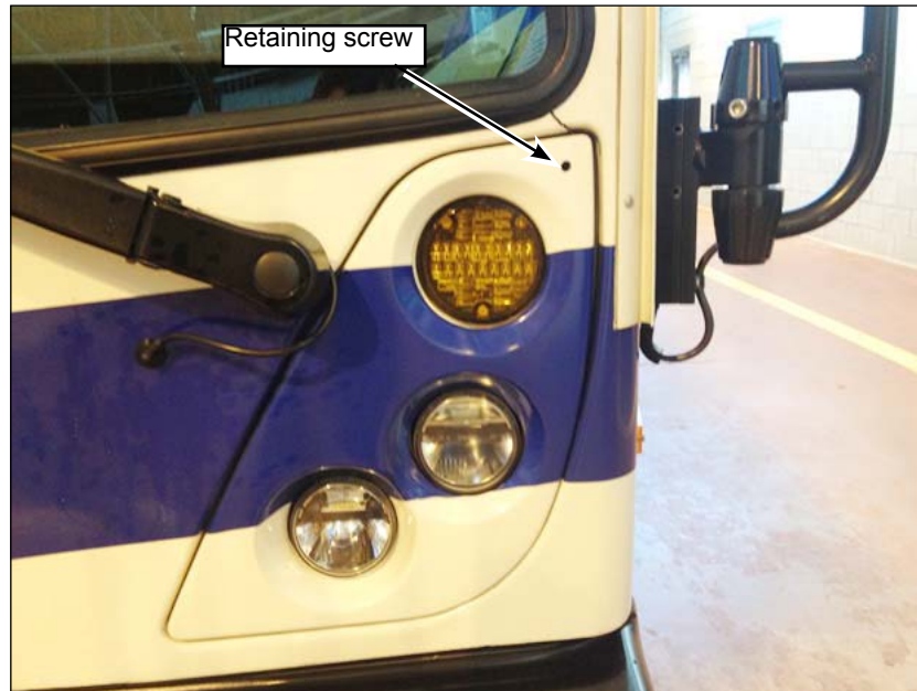
Figure 3 - Remove Headlight Bezel
