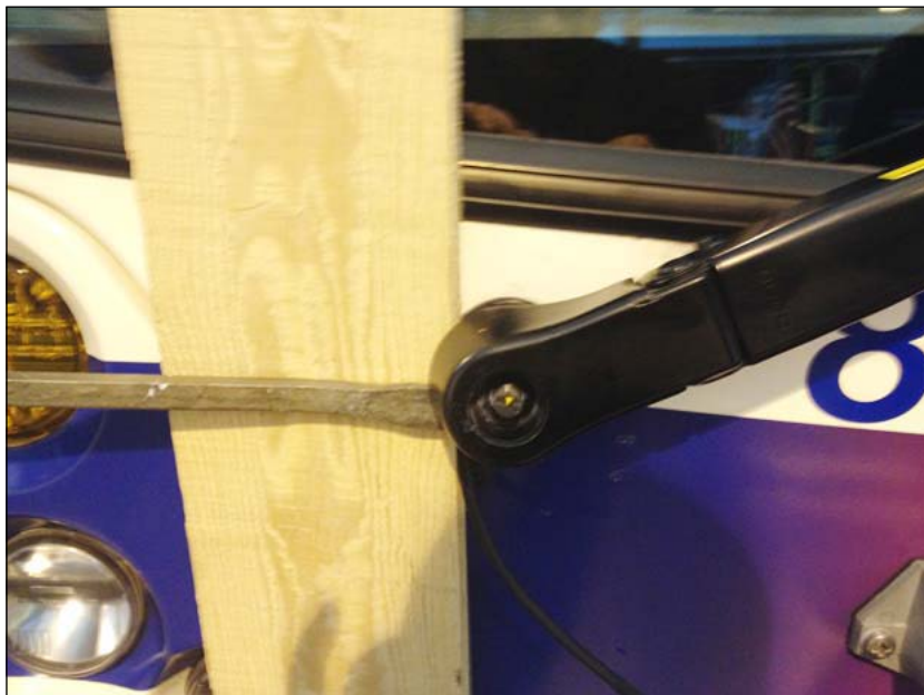
Figure 10 - Remove Wiper Arm
