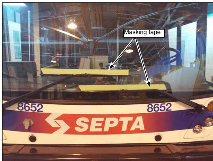
Figure 8 - Place Pieces of Masking Tape
