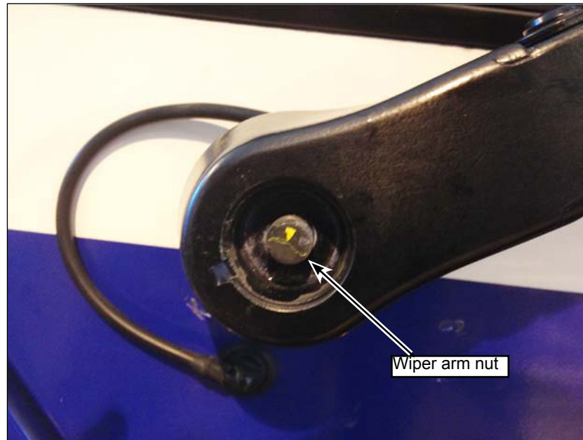
Figure 9 - Remove Wiper Arm Nut and Washer Line
