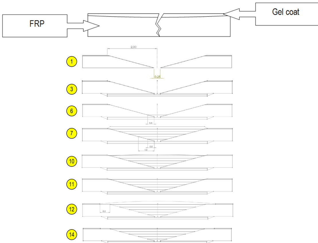
Schematic view of each step for a structural rework of a deep crack
