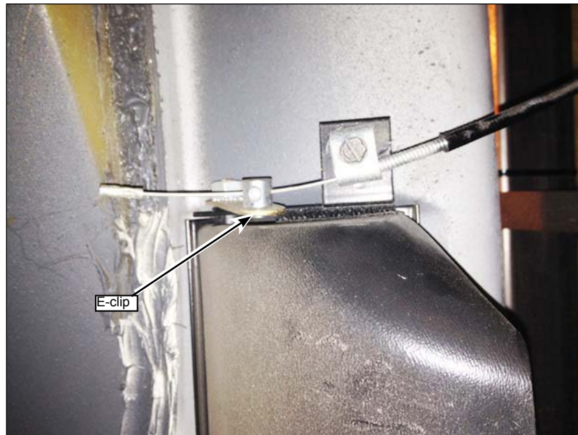
Figure 28 - Install Dash Defroster Cable
