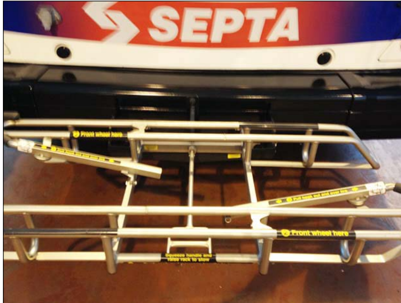
Figure 5 - Lower Bike Rack to Remove Retaining Screws
