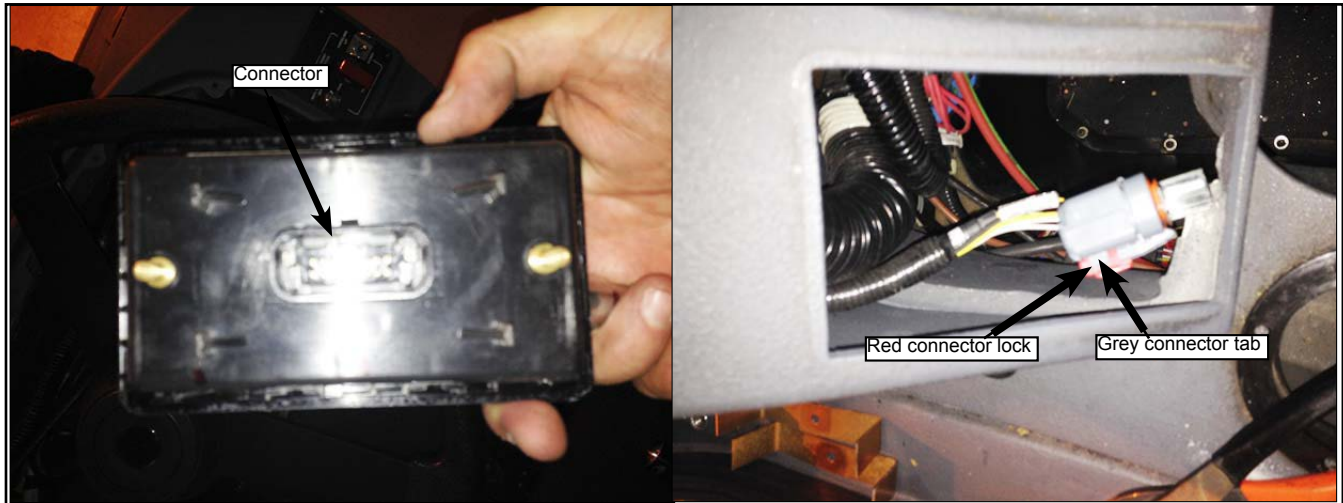
Figure 19 - Remove Connector at Rear of Shift Selector
