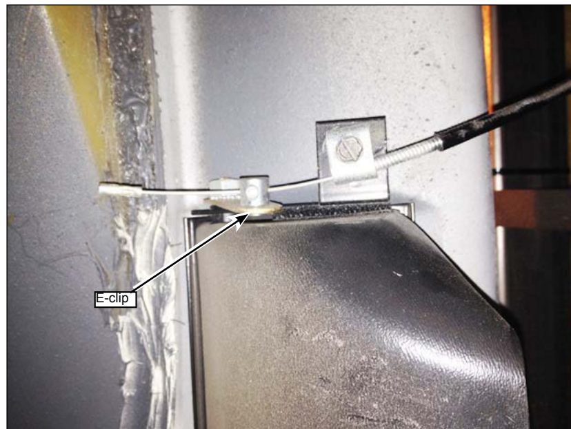
Figure 20 - Remove Dash Defroster Cable
