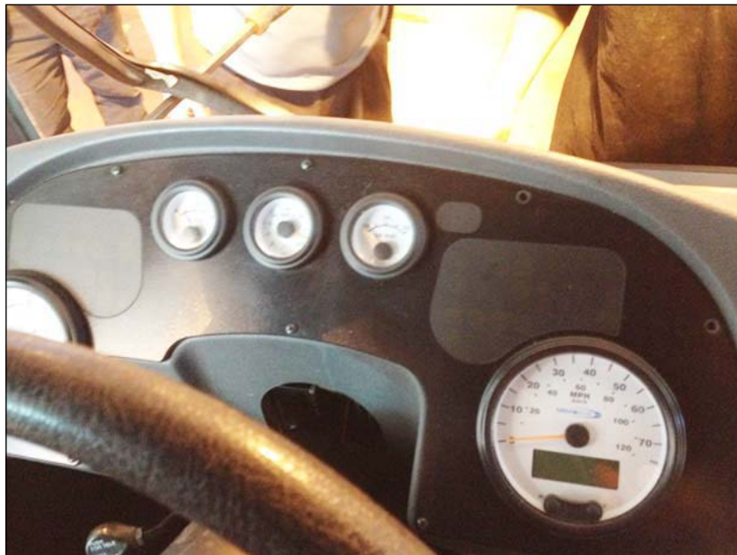
Figure 18 - Remove Dash Screws
