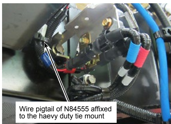
Figure 4 - Installation of Harnesses to the Support Bracket
