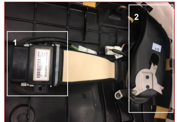
Fig. 3. K900 Climate Control Seat components: 1. TED; 2. Blower motor
