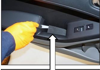
Remove one (1) screw from the door handle pull pocket area of the door panel.
