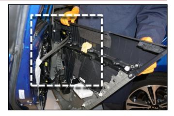
9. Remove three (3) screws securing the window motor to the door module.
