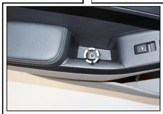
6. Dislodge the bottom portion of the door panel using a non-marring trim panel removal tool.
