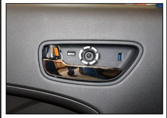
4. Use a non-marring trim panel removal tool to remove the mat from the door handle pull pocket area.
