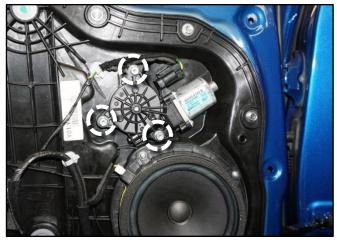
Disconnect the wire harness connector from the window motor and remove the window motor.
