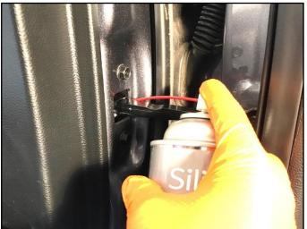
4. Verify operation of the rear doors after lubrication and ensure ease of opening and closing.
