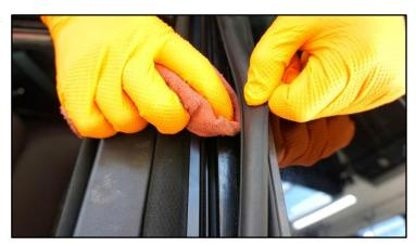
3. Apply a thin bead of adhesive to the weather strip.
