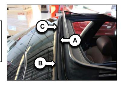
2. Partially remove the affected area of weather strip and clean the contact surface between the strip and sunroof frame using alcohol or a general purpose adhesive cleaner.
