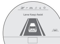
Left: When the LKAS sensor detects the lane traveling in, both lanes are illuminated
