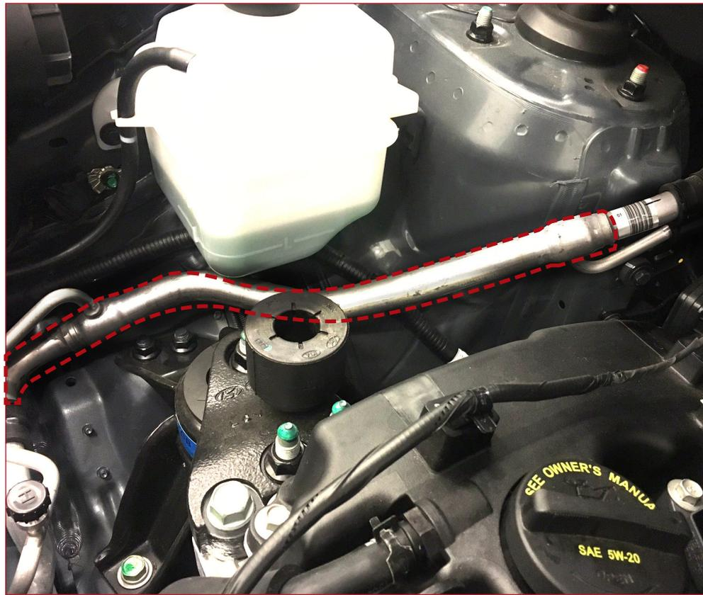
Fig. 1 (left): Inside View of Dual Refrigerant A/C System Line
