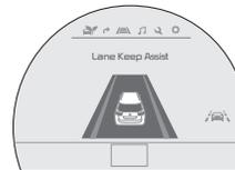
Right: When the LKAS sensor does not detect the lane traveling in the lanes are not illuminated
