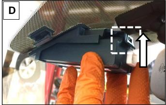
After reattaching the camera, perform the LDWS (MFC) calibration using SST 09890 3V100 by referring to the "Body Electrical System → Lane Departure Warning System (LDWS) → Repair Procedures" chapter in the applicable Workshop Manual on KGIS.
