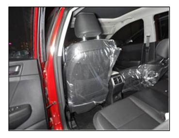
Reposition the front seat back board strap (A) between the side air bag harness and the seat rail (B). Make sure the harness is positioned outboard of the strap. See pictures.
