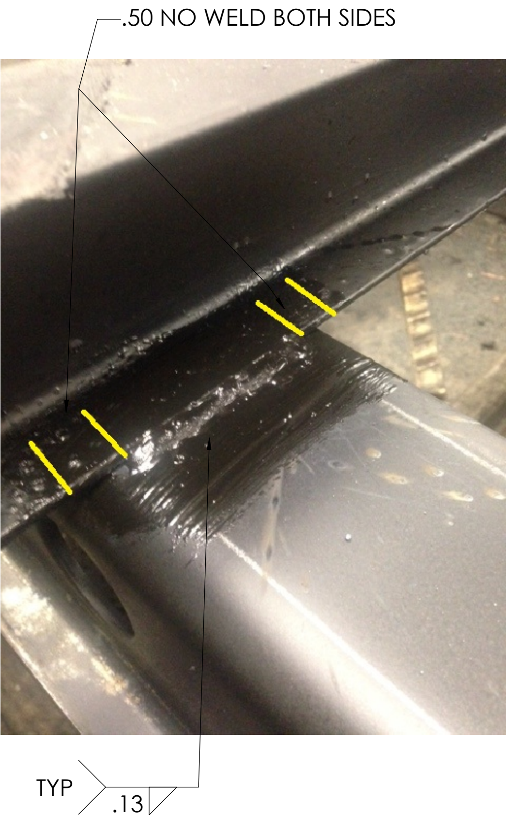
2 CROSSMEMBER TO SLIDER RAIL WELD
