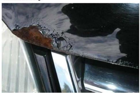
Corrosion may be found on the folded edge of the hood. The corrosion may be found on this edge anywhere around the hood.
