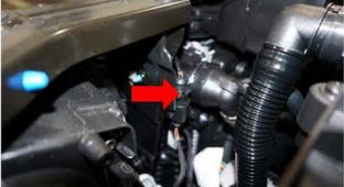
**Step 14:** Check to see if hood latch micro switch is already installed. If so skip this step, If not remove hood latch and install the micro switch into the hood latch.
