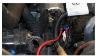
**Step 13:** Remove the red wire from the starter solenoid connector. Insert the red wire from the kit in the connector. Insulate the red wire removed from the starter connector.
