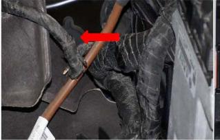
**Step 12:** Pass the remote start harness into the engine bay.
