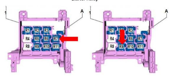
**Step 10**: Unlock starter relay -2- printed with "645" and remove. Located in position R7 shown above. Install relay into the new relay holder in the kit. Insert new relay and relay connector into a free spot in the relay panel.
