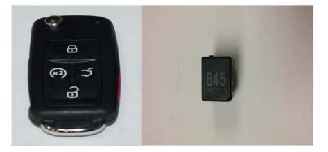
Additional parts required: Key part number 561837202D INF, relay part number 4H0951253A. Vehicles without fog lights, BCM MUST be replaced refer to ETKA for newest part number.
