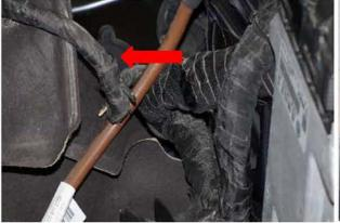
**Step 11:** Pass the remote start harness into the engine bay.
