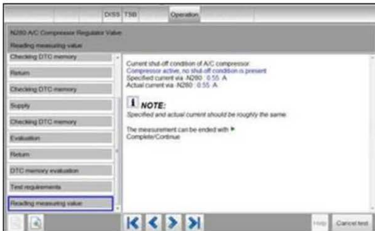
Figure 5. Checking N280 signal value Measuring Value Block.
