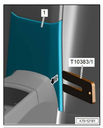
Unclip the center rear panel trim panel <1> with the Wedge Set <T10383/1> in direction of <arrow> and remove.
