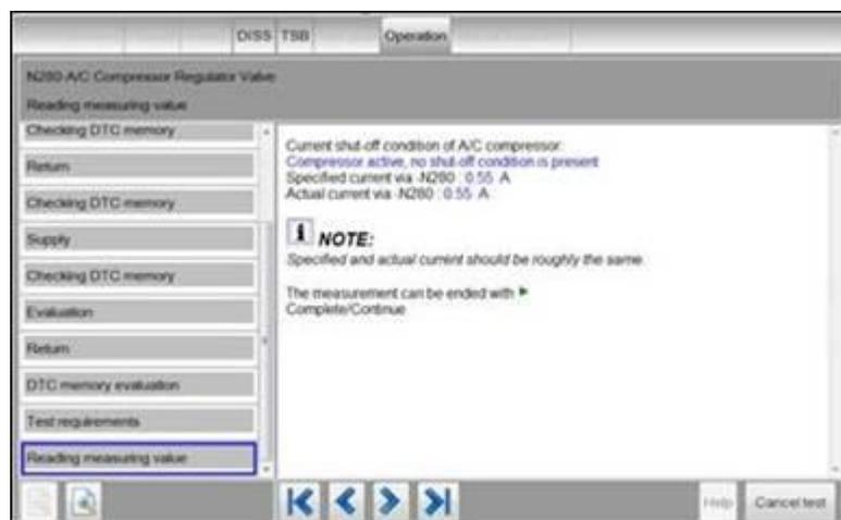
Monitor the measuring value for the air conditioner compressor regulating valve N280 signal (Figure 5).
