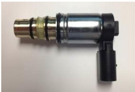
**Figure 1** N280 Refrigerant Regulating Valve
