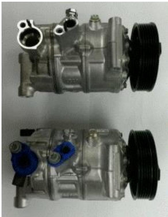
When installing a new compressor transfer the compressor shipping caps to the original compressor as shown in Fig 18.
