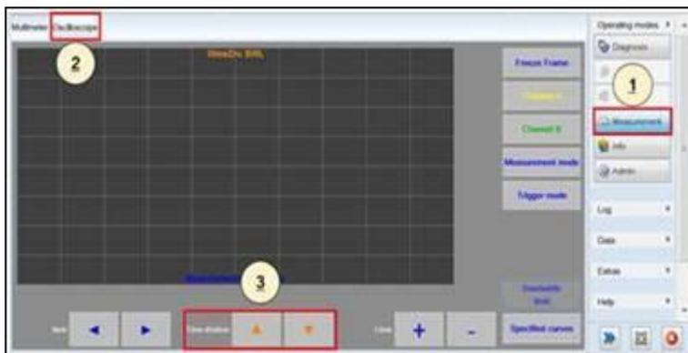
Go to Operating Mode "Measurements" to check the N280 signal from the control module.
