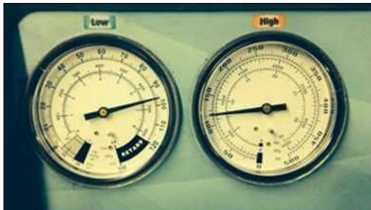
**Figure 6.** Equalized pressure condition. No pressure generated from compressor.
