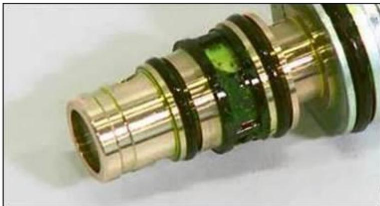
Should severe contamination be found at the valve filter screen (Figure 15) and A/C compressor replacement becomes necessary, ensure that the refrigerant circuit is flushed in the course of repair.
