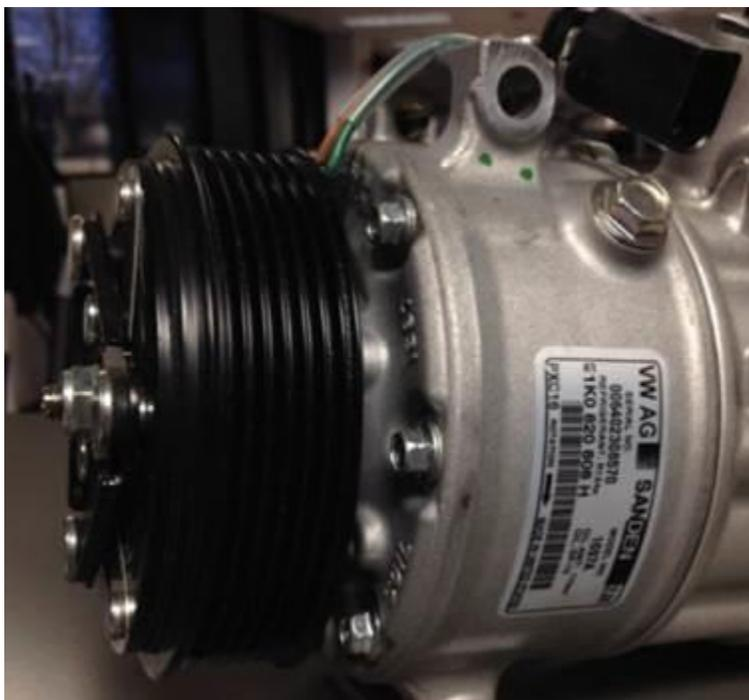
**Figure 8.** MY2016 AC compressor with clutch (Sanden)
