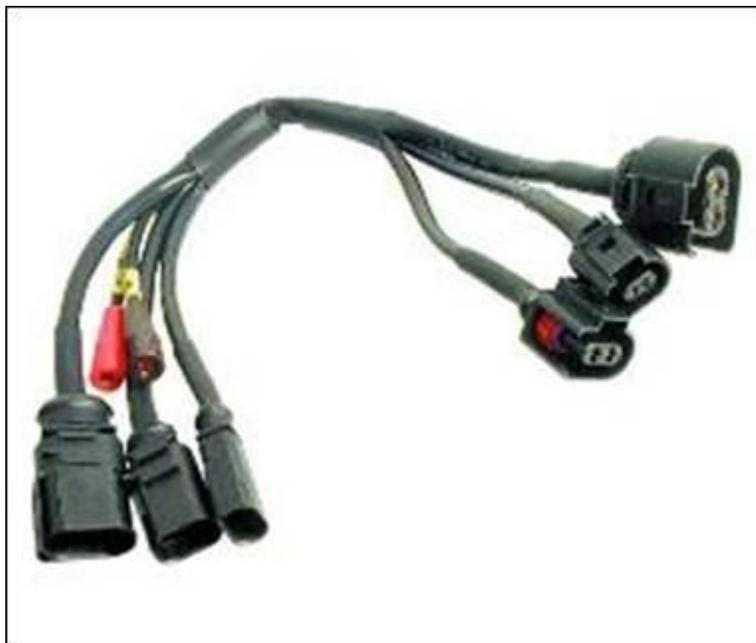
Shut off the engine. Connect the breakout harness VAS 5256 (Figure 9) between the N280 valve and its connector.
