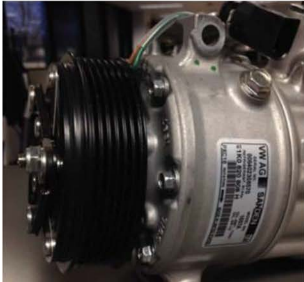
Figure 8. MY2016 AC compressor with clutch (Sanden)
