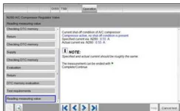
Figure 5. Checking N280 signal value Measuring Value Block.
