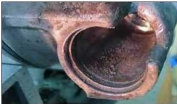
Figure 14. Corrosion in the N280 valve bore.
