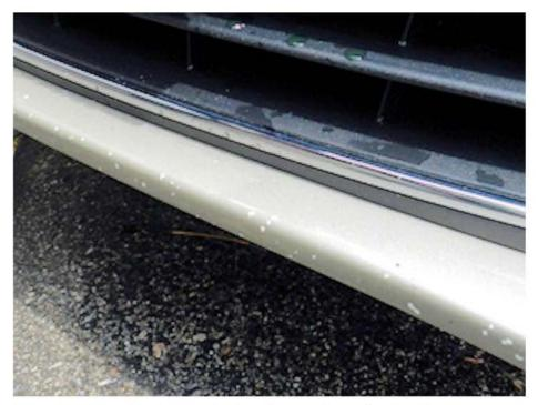
Extensive stone chipping may be found across the entire front bumper cover. Damage may be centralized to the bumper cover with no paint chipping anywhere else on the vehicle.
