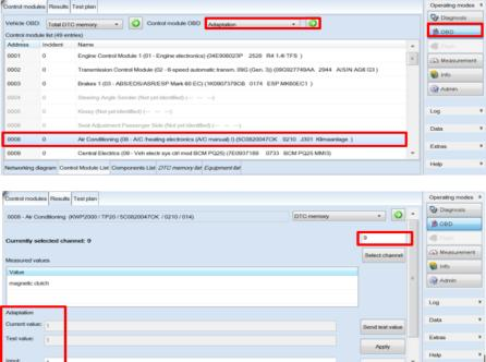
The wiring to the N280 from the AC clutch relay does not provide feedback to the AC controller for open or shorted wiring. Always check the AC shut off codes in ODIS measured values and the system is fully charged before starting any diagnosis.
