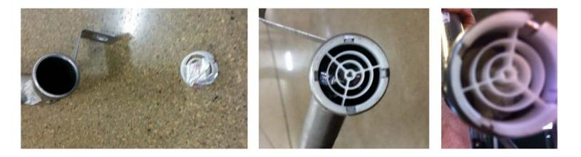
If the anti syphon device is dislodged it will cause the fuel flow to be disrupted and can cause shut off problems (as per the example below):
