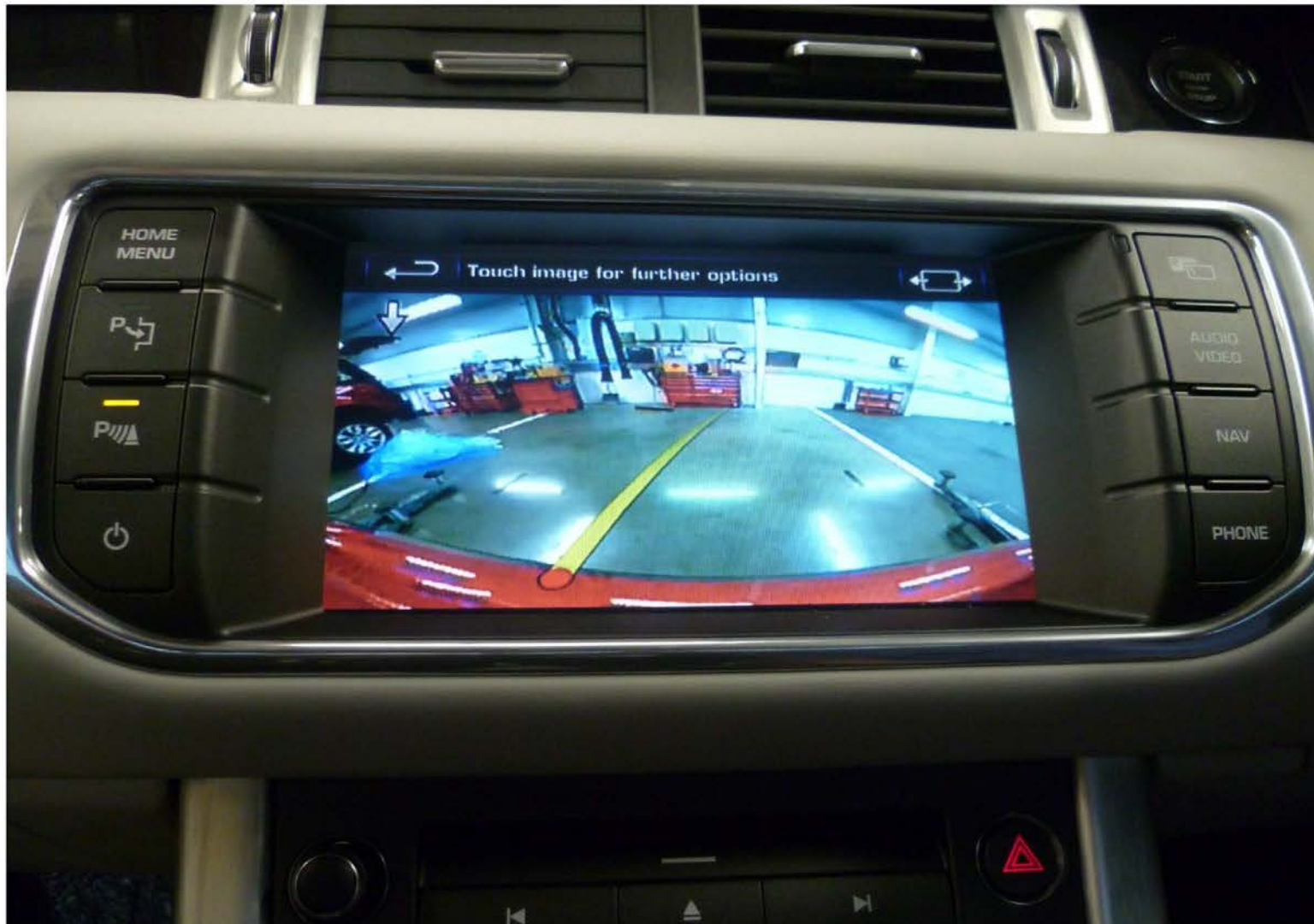
High Line Reverse Camera View : Tailgate Finisher shown with a line of curvature
