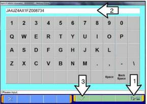
b. Click the icon in the lower RH corner of the screen to have MUT—III automatically read the VIN.
