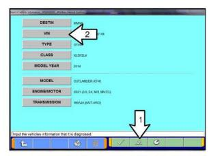
a. If the VIN or vehicle description displayed does not match the vehicle you are working on, click the eraser icon at the bottom of the page to erase vehicle data. Then click the "VIN" button.
