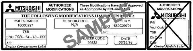
NOTE: The Control Module Label is NOT used for this reflash. It should be discarded.
