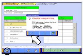
If the message seen at left is displayed, the ECU software is already at the most current level. Do not continue with the reprogramming procedure. This TSB does **not** apply.
