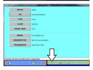
c. Confirm all data matches the vehicle, then click the check mark at the bottom of the page.
