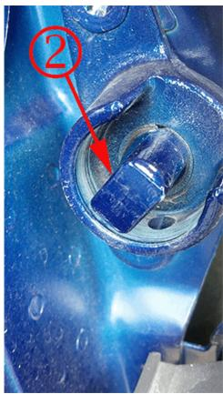
4. If the tailgate has additional closing effort, inspect for improper lubrication at the left tailgate hinge bushing. The left tailgate hinge should be lubed during scheduled maintenance to prevent increased operating effort or noisy operation. Refer to the latest version of bulletin 13-08-66-001 for more information.
