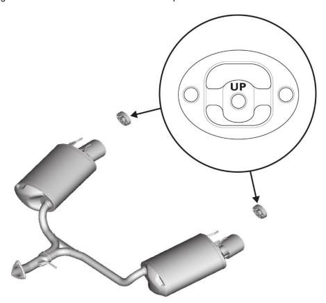
To address this issue, make sure both rubber exhaust hangers are properly installed.
