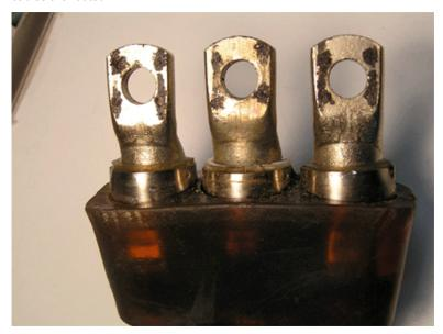
This is signs of pitting/arching. These should be replaced. Minor pitting can be cleaned up and the cables reused.
